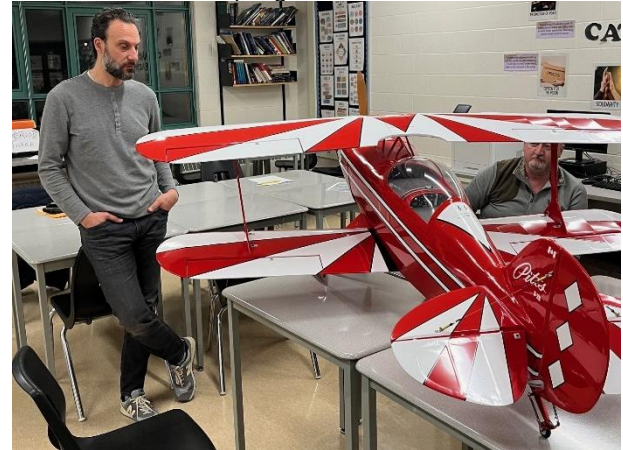
Paul shows his spectacular Pitts Special at the AGM Hangar 9 Pitts Special S-2B - 1/3 scale, DLE 60 Twin Spektrum Equipment: PowerSafe RX and Synapse gyro Custom 3D printed cockpit interior 71.6" Wingspan, 20.2lbs Weight
