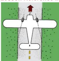
If a model is hard to keep tracking straight in take-off, it could be caused by incorrect landing gear alignment. For <u>tail draggers</u>, main gear wheels should toe in slightly toward the center line. Two to 5 degrees is usually enough. However, for <u>tricycle gear</u>, wheels should toe out slightly.
